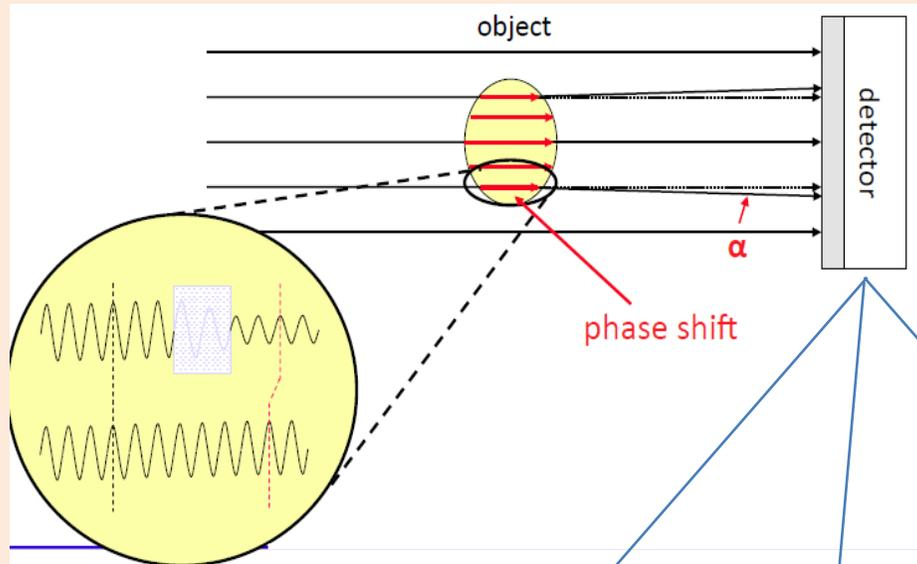
Most sensitive to abrupt changes in the refractive index: gives **edge enhancement**.
