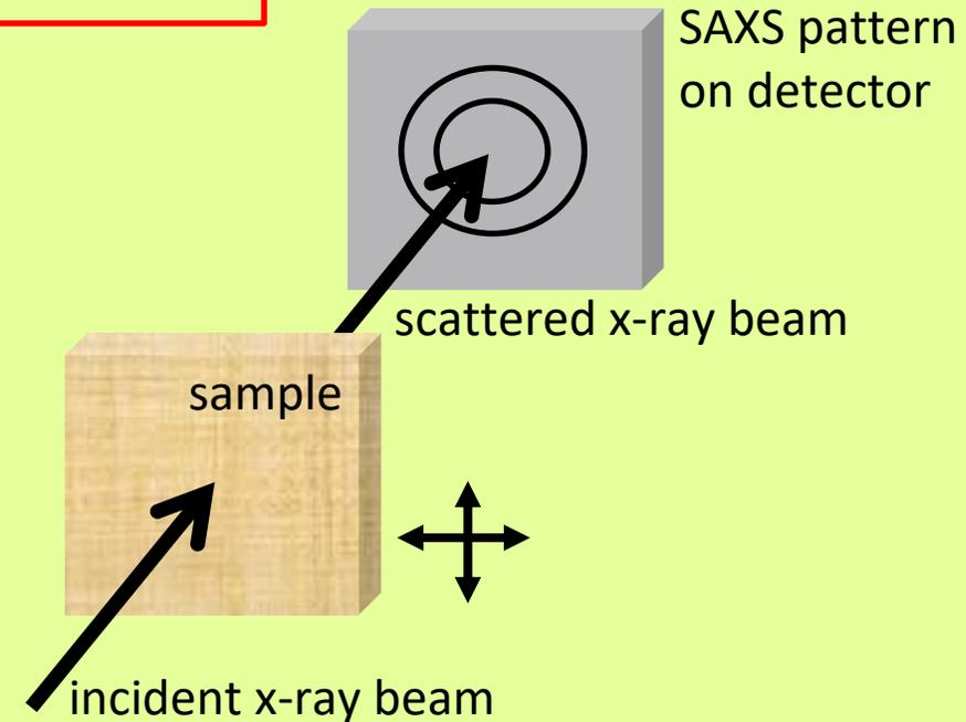
X-ray beam size  $\rightarrow$  real-space resolution ( $\approx 1 \times 1 \mu\text{m}^2 - 50 \times 50 \mu\text{m}^2$ )
