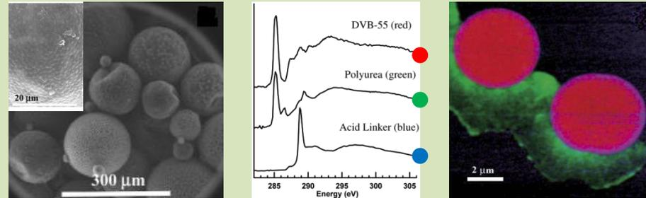
Composite Tectocapsules Containing Porous Polymer Microspheres
