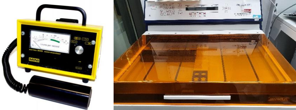
Figure 5 A radiation protection instrument (left) shall be available for measuring contamination of gamma (ex. Cr-51) or high-energy beta (ex P-32) emitters. A beta counter (right) shall be available for measuring contamination of low-energy beta emitters (ex. H-3, C-14 and S-35).
