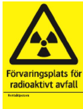
Figure 10 Mandatory storage sign for radioactive waste. Please note that the name of the assistant shall be specified, too.
