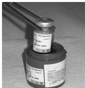
Figure 6 Pliers/tweezers shall be used when handling gamma or high-energy beta radiation.
