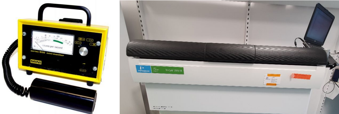
Figure 5 Radiation protection instrument to the left and liquid scintillation counter to the right.
