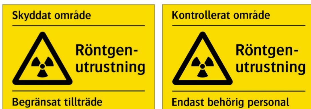
Figure 2 Sign for a supervised area (left) and a controlled area (right) respectively.
