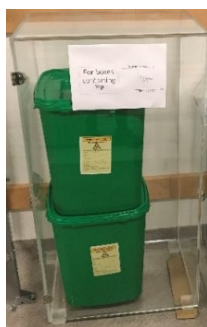
Figure 7 Green containers might require extra shielding, e.g. plexiglass for high-energy beta emitters (ex. P-32) or lead (ex. Cr-51).
