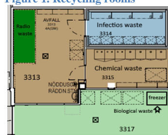
Figure 2. Hazardous waste rooms
