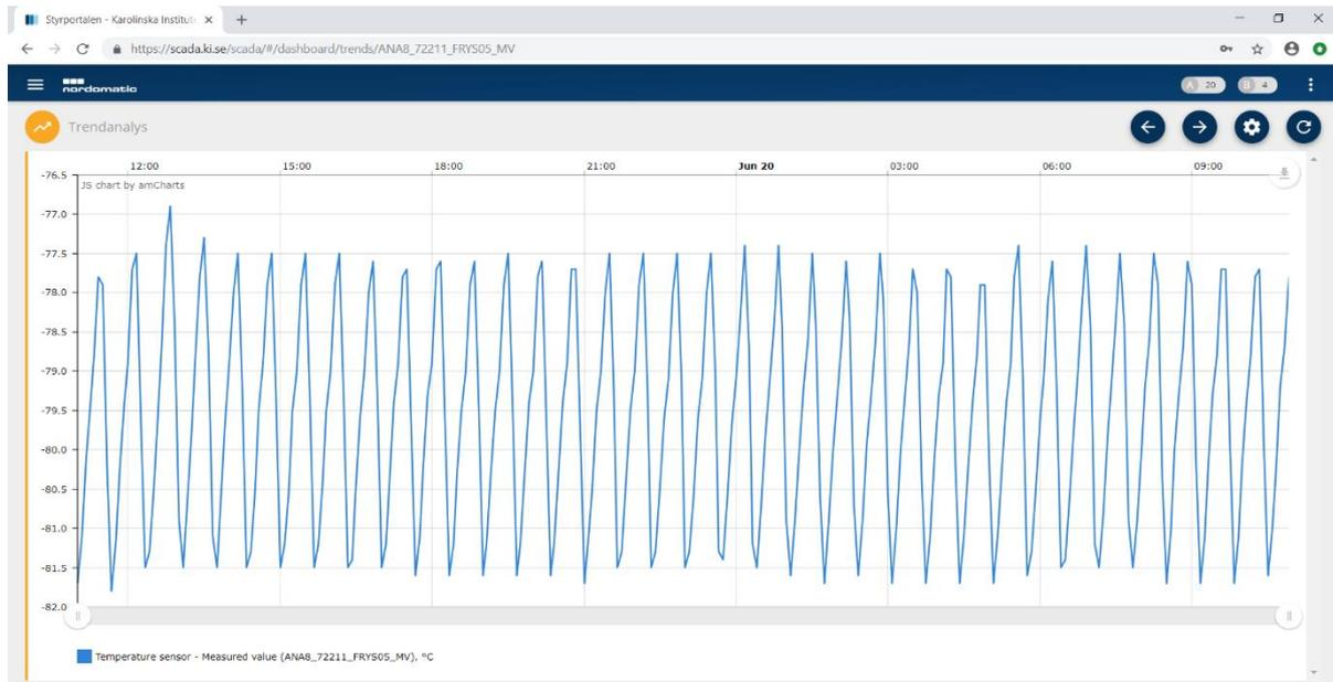
Here you can view the temperature reading of the Pt-100 sensor with a sampling rate of 5 minutes.
